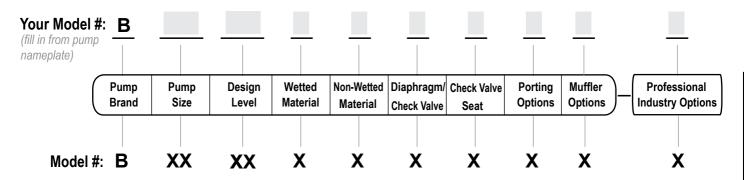
**Pump Brand Non-Wetted Material Options Porting Options** SeficoPower **NPT Threads** Α Aluminum Ν Χ **Unpainted Aluminum** В **BSPT Threads** R Threaded Flange **Pump Size** Welded Flange 1 1/2" 15 **Diaphragm/Check Valve Materials** 1 Santoprene/Santoprene 2 PTFE-Santoprene/PTFE **Muffler Options Design Level** G **Body Connected Muffler** PTFE-Neoprene/PTFE 01 Design Level M Santoprene/PTFE
